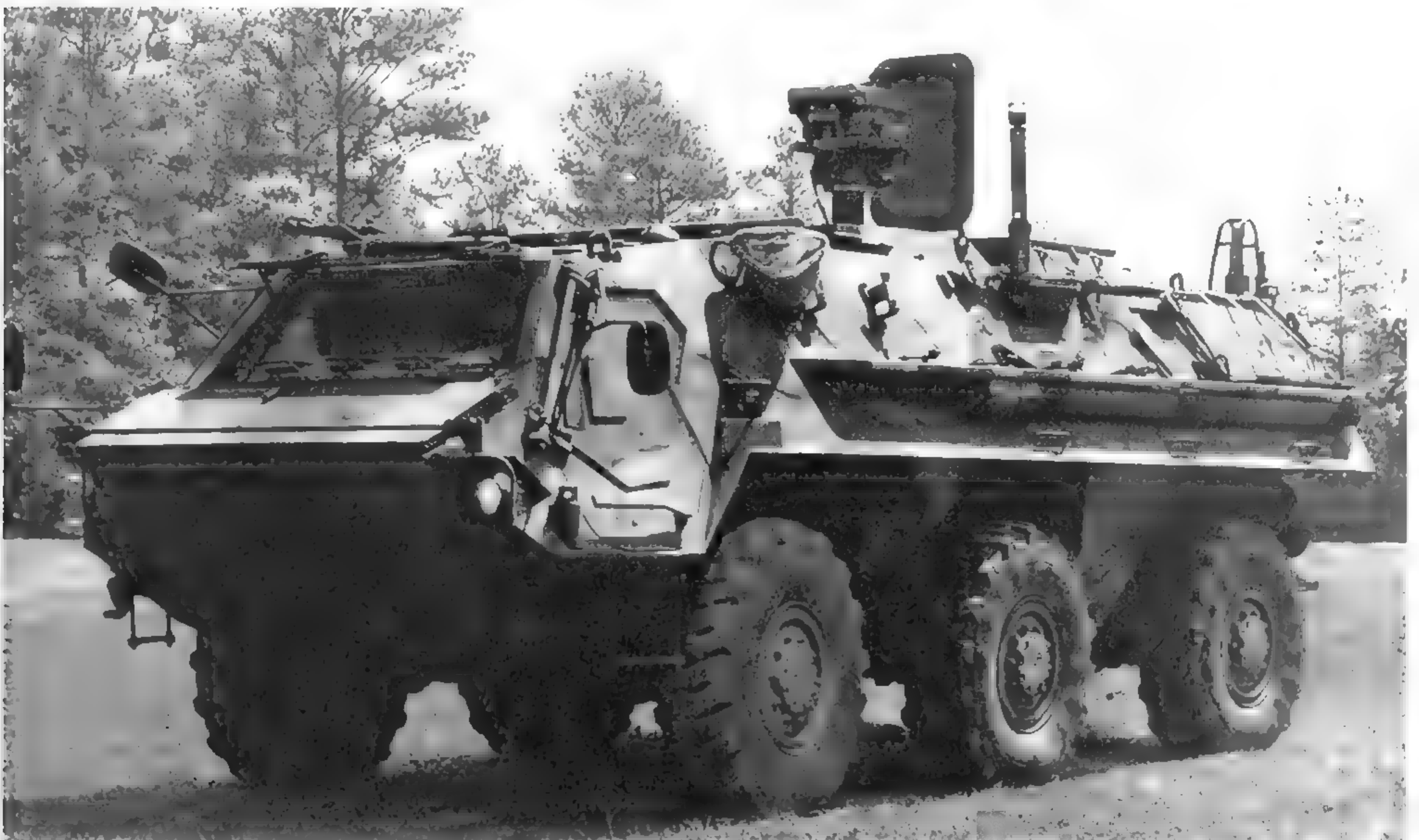
The M93 Fox is the U.S. version of the German Fuchs NBC vehicle. The base vehicle is the Thyssen Henschel TPz1 armored personnel carrier, which was adapted to a NBC detection role by German forces, then adopted by the U.S. military. (U.S. Army photo)
